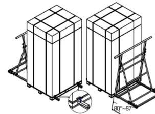
2. Pass the forearm of the anti-tilting bracket through the pallet, insert the two bolts into the front round hole of the anti-tilting bracket, and adjust the support angle of the anti-tilting bracket so that the angle with the ground is between 80° and 87°.
