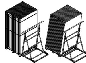
3. Remove the packing belts and carton (the cardboard on one side of the anti-tilting bracket can be retained), leaving only 1 or 2 internal belts, then carefully push the modules so that they rest diagonally against the anti-tilting bracket.
