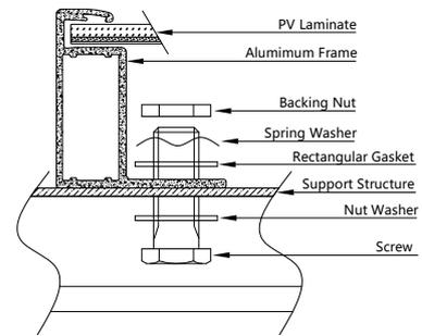
Figure 11: Detail of a bolt installation attachment
