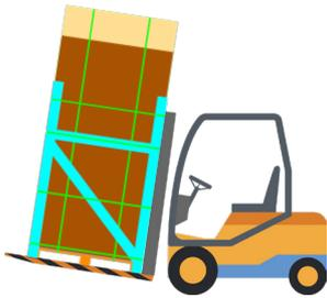
2. Safety ropes are required to secure the modules to the forklift with a tensile strength greater than 2000 kgf.
