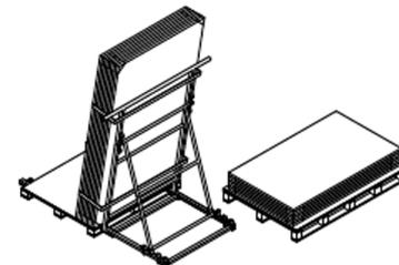
4. Two people work together to carry the modules one by one, if there are any left over, secure the remaining modules to the anti-tilting bracket with tie-downs or place them flat on a pallet (no more than 20 pieces per pallet).
