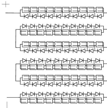
Figure 7-2: Electrical circuitry of cells and bypass diodes
