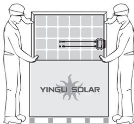
Figure 3: Removing PV modules from a pallet
