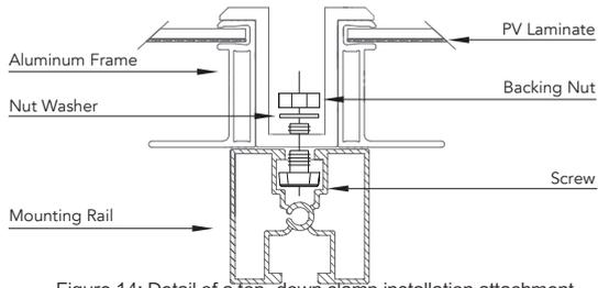
Figure 14: Detail of a top-down clamp installation attachment
