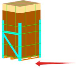
1. Forks enter in the direction of the long side of the pallet, close to the pallet and prohibit slamming against the modules.
