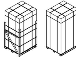
1. Place the package on the flat working ground, cut the packing belts and remove the wooden brackets.
