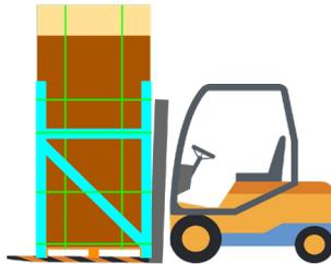
3. When placing it, need to wait for the packing box to be stable before untying the safety rope.
